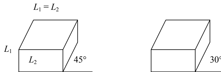
Fig. 11.10 Two Cubes Cavalier Projection
